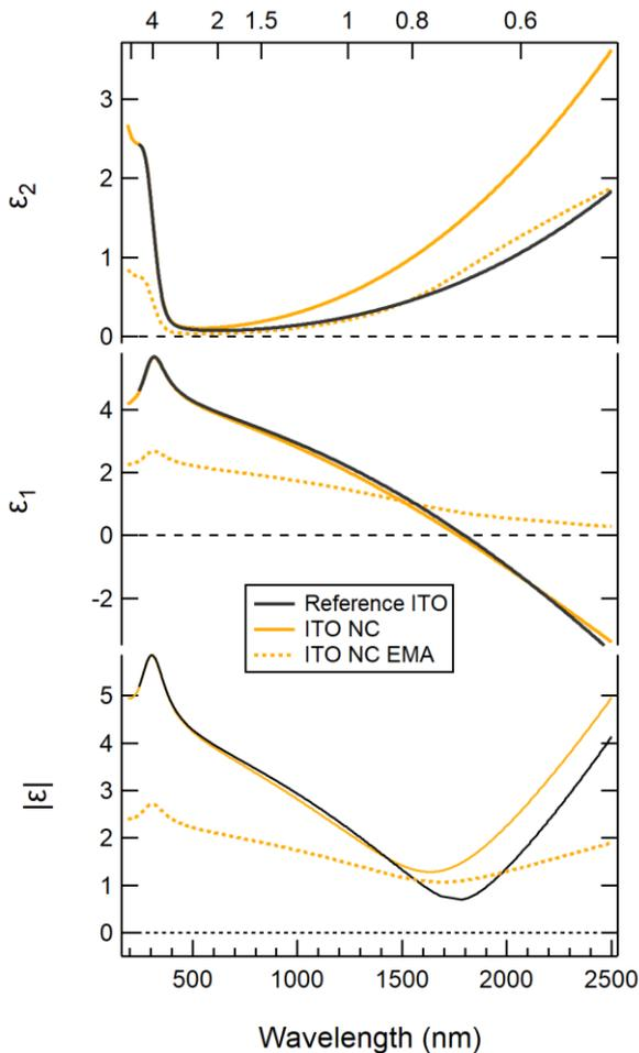
**Figure 4.** Top panels: real and imaginary parts of dielectric functions of the ITO reference film (black line), of the ITO scaffold in the NC films (solid orange line) and of the whole ITO NC film (dashed orange line). Bottom panel: modulus of the respective dielectric functions.
