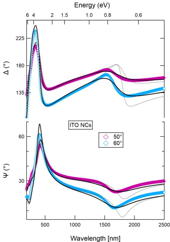
**Figure 3.** Variable-angle SE spectra of a nanoporous ITO NC film on SiO<sub>2</sub>/Si (markers). Best fit of the experimental data obtained allowing a variation of the free-electron contribution to  $\epsilon$  (solid black lines) or using the bulk values for  $\epsilon$  (dotted lines). See text for details.
