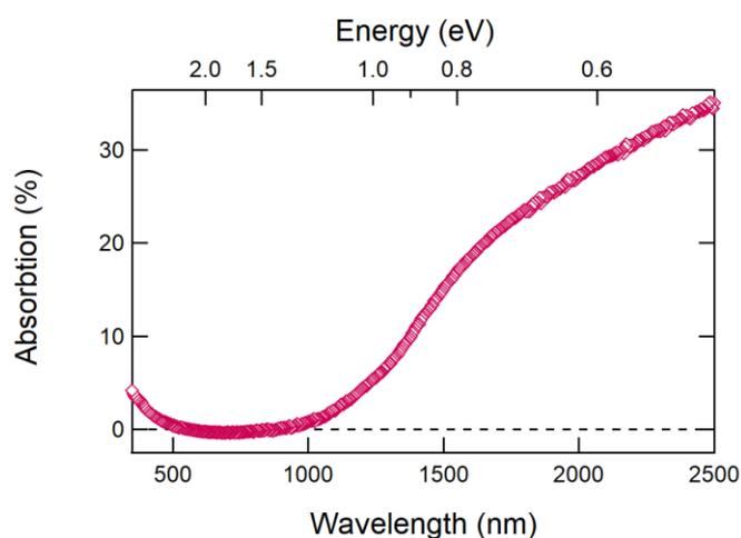
**Figure 5.** Absorption of the ITO Ncline film.
