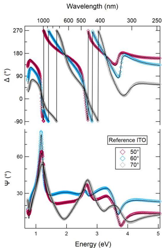
**Figure 2.** Variable-angle SE spectra of the reference ITO film on SiO<sub>2</sub>/Si (markers). Best fit to the experimental data (lines).
