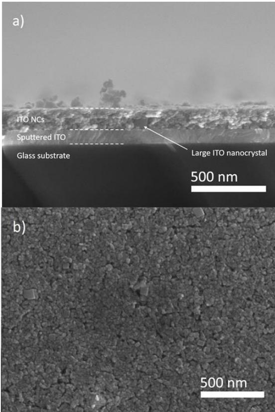
**Figure 1.** Scanning electron microscopy cross-section (a) and top view (b) of a NCs-based ITO film. A clear difference in morphology is evident with respect to the commercial bulk ITO sputtered film on which the ITO NCs film is deposited.
