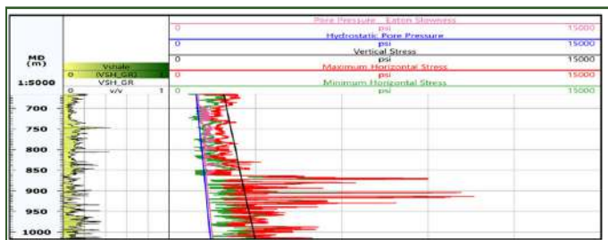
Figure 6: Horizontal stresses of Dammam formation predicted according to the poro elastic horizontal strain model.
