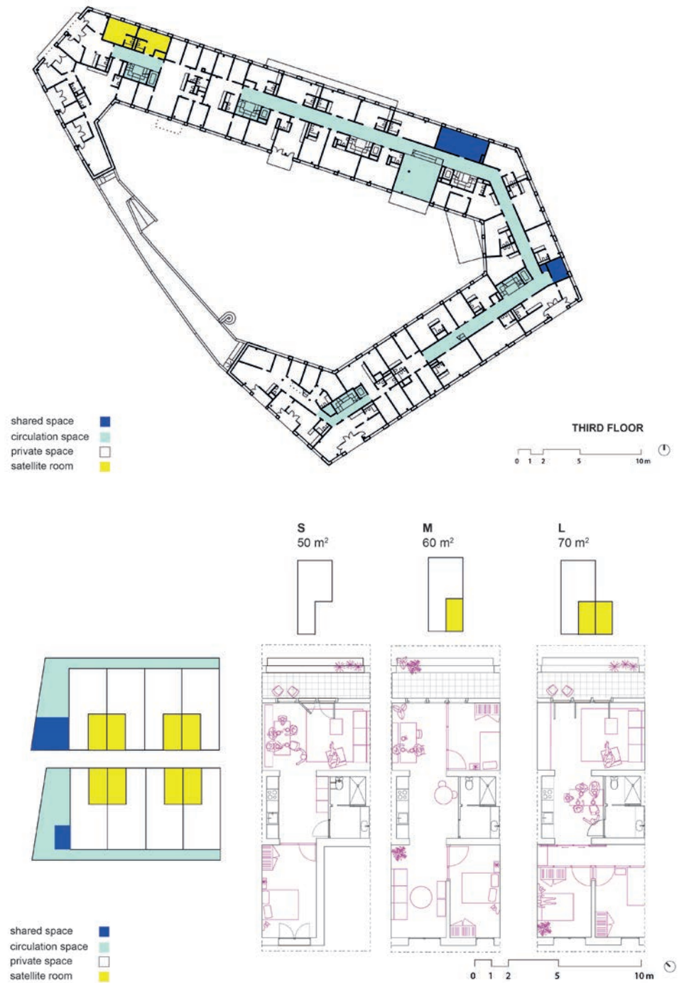
Figure 4. La Balma, Barcelona, Spain, Laco and laboqueria, 2017-2021. Modular system of flats, changing from S to L typologies with the addition or removal of satellite rooms.
