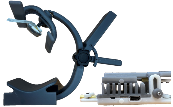
Fig. 2. 3D printed enclosures realized for the blood pressure device. Support containing the elbow's sensor (left). Finger clip holding the thumb sensor (right).
