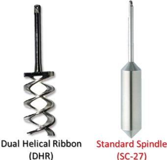
Figure 19. The dual helical ribbon (DHR) and the standard coaxial geometry (SC-27) used in this study
