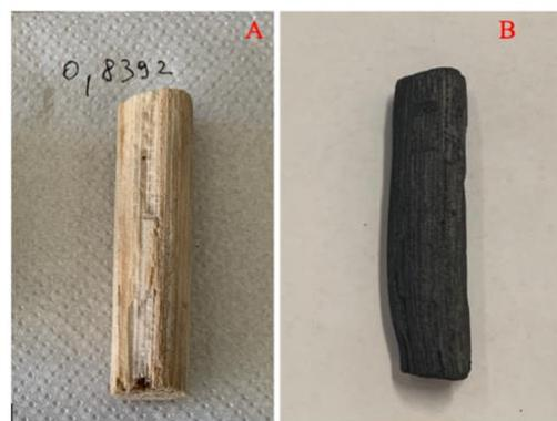
**Fig. 3.** Example of: A) pre pyrolyzed sample; B) pyrolyzed sample
