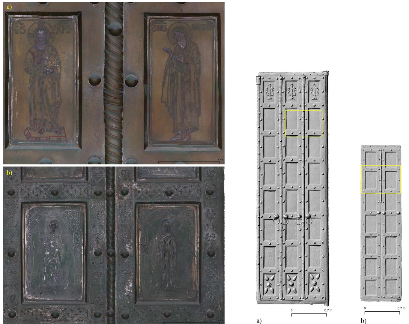
Fig 3. Basilica di San Marco, Venice, Italy. Orthophoto detail, shaded Digital Surface Model. a) Main door, right leaf, plates E2 (left) and F2 (right). b) Door San Clemente, left leaf, plates A2 and B2.
