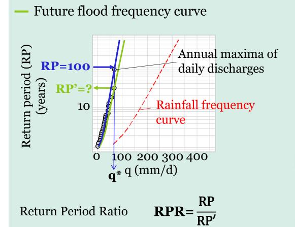
Right-shift of the flood frequency curve → Increase of the frequency of exceedance of the current 100year Flood (RPR>1)
