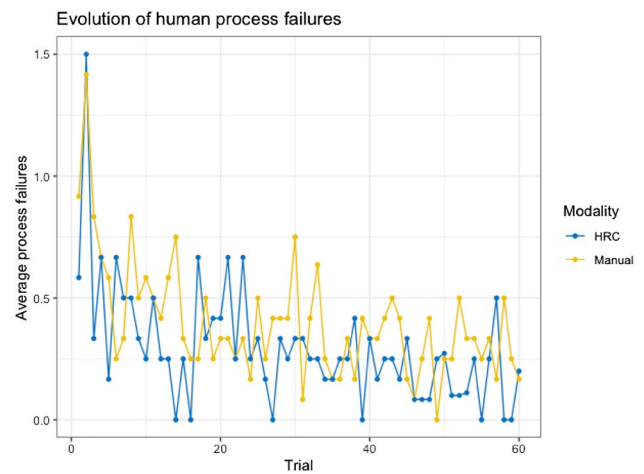
Fig. 5 Evolution over trials of average human process failures for both HRC and Manual modalities
