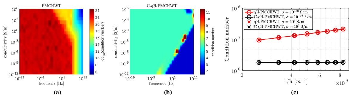
**Fig. 1.** Condition number of (a) the PMCHWT formulation (in logarithmic scale) and (b) this work. (c) Condition number as a function of the inverse mesh refinement parameter  $h$ . The geometry is a sphere with radius 10  $\mu\text{m}$ .
