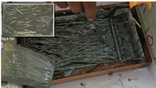
Fig.3 Hand-layup of S2, S3 samples
