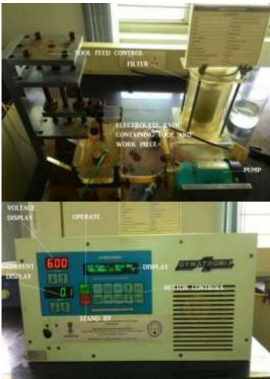
Fig. 1: Micro ECMM setup and pulse rectifier
