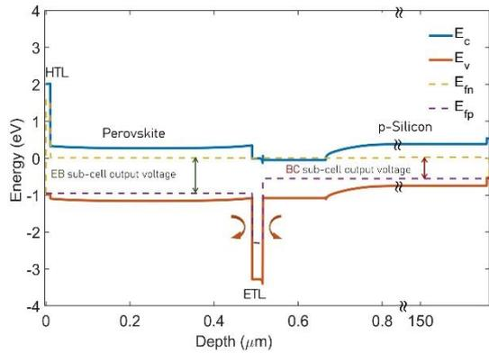
**Figure 2:** Energy band diagram of the  $p\text{-}n\text{-}p$  3T-HBT with each junction biased at maximum power point. The dashed yellow and pink lines are the electron and hole quasi-Fermi levels, respectively.
