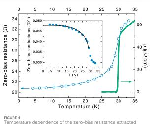
Temperature dependence of the zero-bias resistance extracted from the curves in Figure 3G (blue hollow circles, left scale) compared to the resistivity of the same crystal (solid green line, right scale). The inset shows the zero-bias conductance (filled blue circles), that follows the same temperature dependence of the gaps up to 29 K (solid black line).
