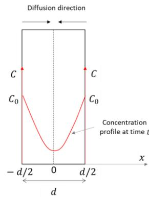
**Figure 4.** Concentration profile across the sample. Modified after [47].
