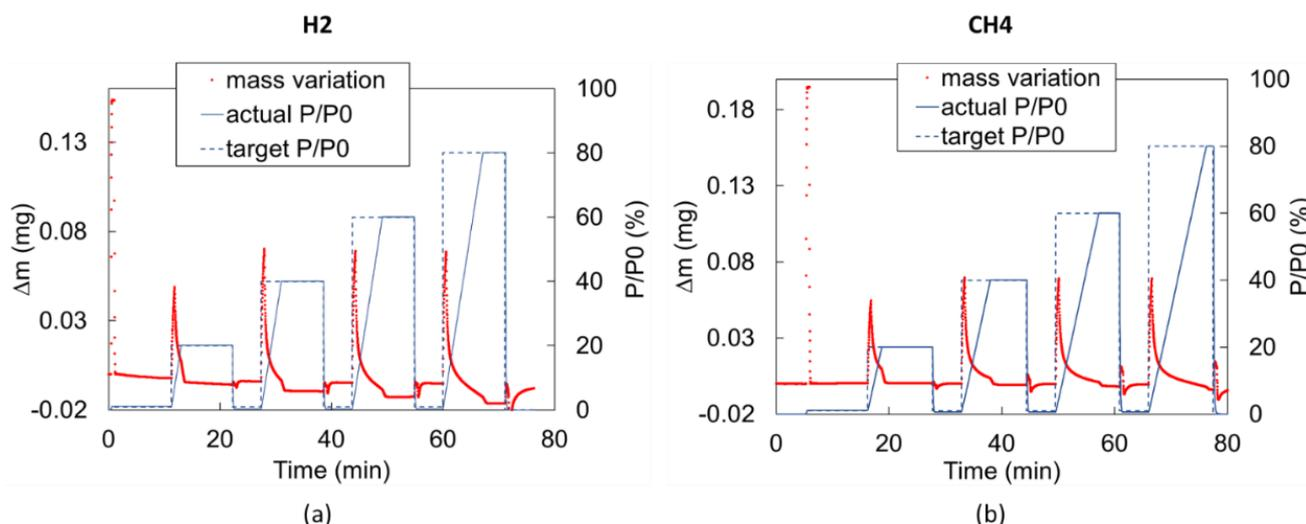
**Figure 6.** Measured mass variation in time during (a) H<sub>2</sub> blank run and (b) CH<sub>4</sub> blank run. In both cases, a significant overshooting effect is observed.
