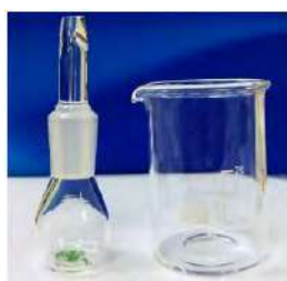
Figure 1. Pycnometer used for the density measurements.
