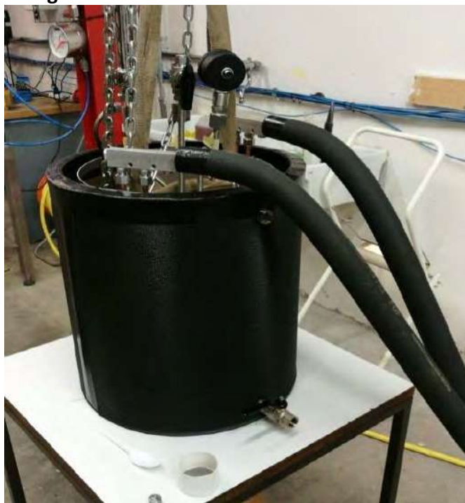
Figure 2. Reactor in the thermostatic bath.
