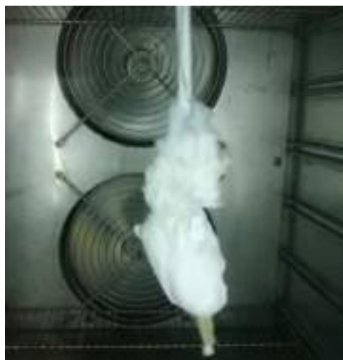
Figure 4. Picture of the electric heating wire rolled up with the cotton candy.
