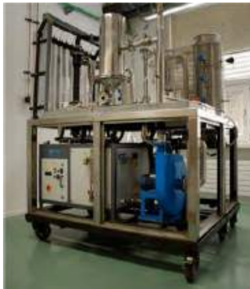
Figure 1. The small-scale biomass gasifier that is installed in the Bioenergy Laboratory of the Free University of Bozen-Bolzano [35].
