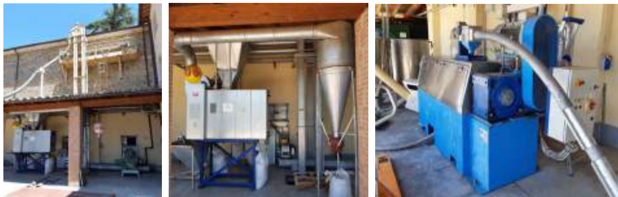
Figure 1. The seed storage, transportation, sifting section (left); sieve (center); the milling machine (right).
