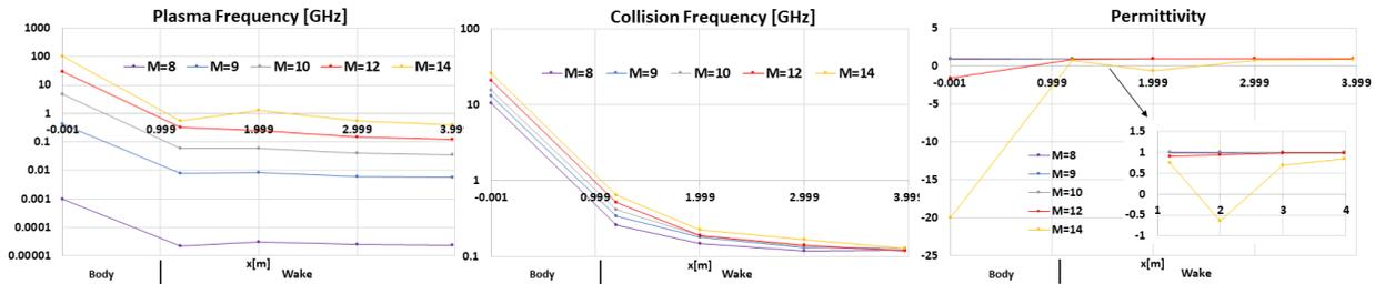
Figure 2. Maximum plasma and collision frequencies, and minimum real part of permittivity at 30 km altitude.
