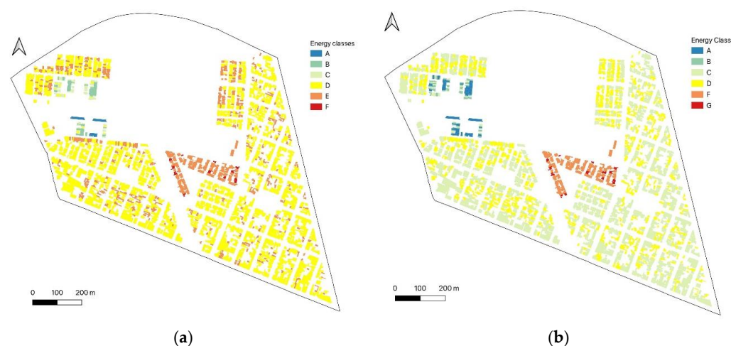
Figure 7. Energy classes after retrofitting interventions in district CD-3: (a) window substitution; (b) thermal insulation of roofs.
