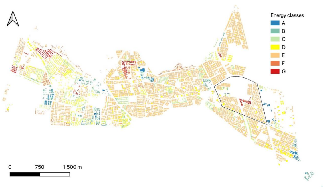
Figure 6. The energy classes of residential buildings in Renca according to Chilean climate zone 3.
