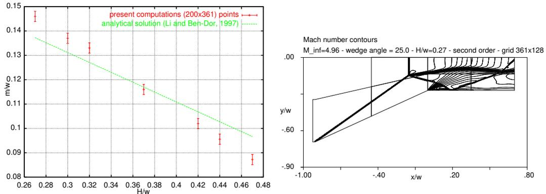
**Fig. 4.** Left: effect of  $H/w$  on the normalized Mach stem height  $m/w$  for Mach 4.96 and  $\delta = 25^\circ$ . Red bars: numerical results (the error bar represents the dimension of one cell in the direction normal to the symmetry axis). Green line: theoretical prediction (from figure 15 of [10]). Right: the Mach reflection configuration for  $H/w = 0.27$
