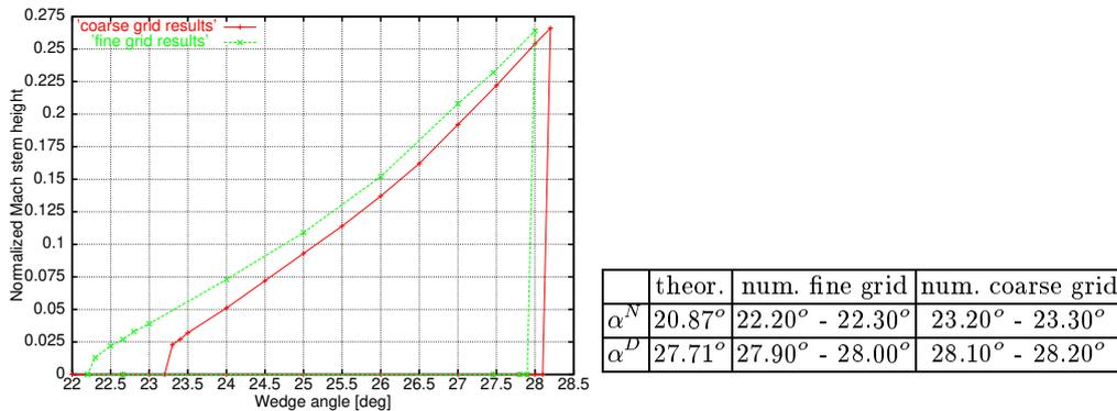
**Fig. 3.** Numerical hysteresis curves for Mach 4.96 and  $H/w = 0.42$ . The red line refers to the coarse grid (181x100), the green line to the fine grid (361x200). Theoretical and the numerical angles  $\alpha^D$  and  $\alpha^N$  for  $M_\infty = 4.96$  and  $H/w = 0.42$ .
