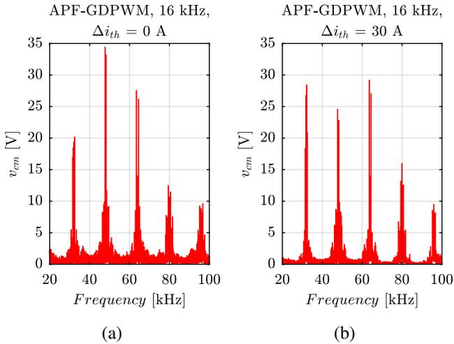
Fig. 10. High frequency common mode voltage injection with  $f_{sw} = 16$  kHz and APF-GDPWM. (a) Hysteresis selector disabled (null  $\Delta i_{th}$ ). (b) Hysteresis selector enabled and  $\Delta i_{th} = 30$  A.
