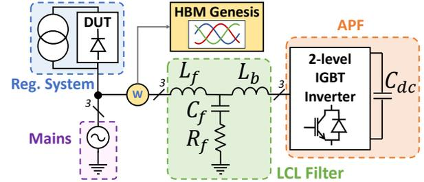
Fig. 11. Scheme of power losses measurement setup.
