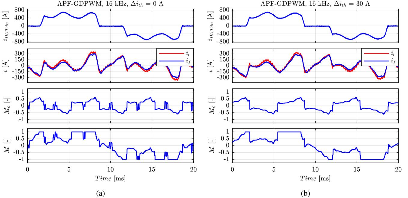
Fig. 9. APF steady-state operation with  $f_{sw} = 16$  kHz and APF-GDPWM in case of hysteresis selector disabled (a) and enabled with  $\Delta i_{th} = 30$  A (b). From top to bottom: current absorbed by the rectifier  $i_{DUT,in}$ , line and grid-side LCL filter current  $i_l$  and  $i_f$ , zero sequence modulation index  $M_c$  and phase modulation index  $M$ .
