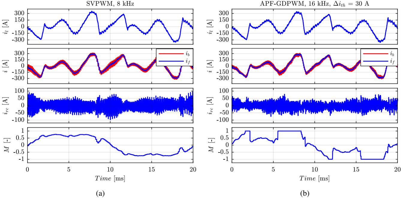
Fig. 12. APF steady state operation in case of SVPWM at  $f_{sw} = 8$  kHz (a) and APF-GDPWM at  $f_{sw} = 16$  kHz with  $\Delta i_{th} = 30$  A (b). From top to bottom: line current  $i_t$ , APF output current  $i_b$  and grid-side current  $i_f$ , RC filter current  $i_{rc}$  and phase modulation index  $M$ .
