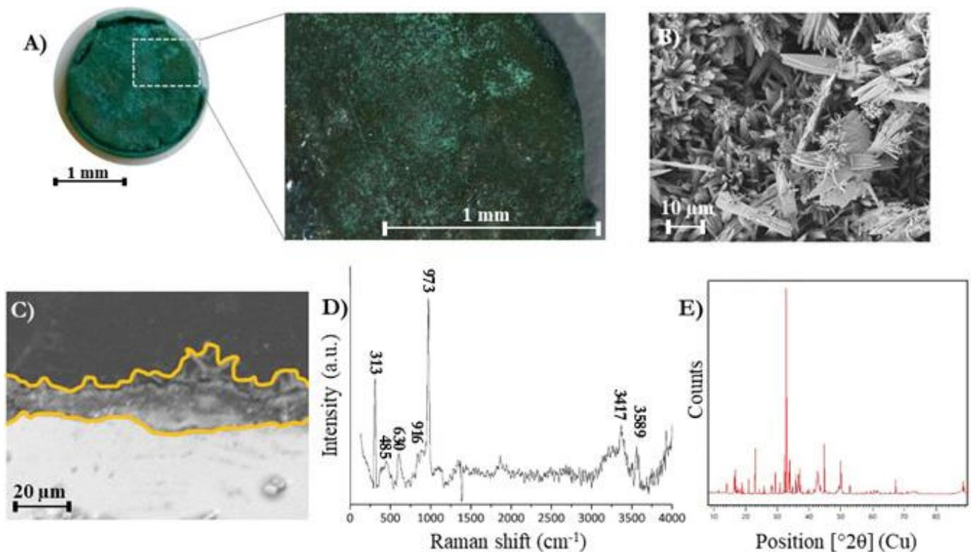
Figure 3. Obtained results on CuSn6Pb4 alloy sample immersed in CuSO<sub>4</sub> solution 50 mM for 15 days. In particular, A) high-quality image of the sample and superficial enlargement, B) FESEM image of the surface morphology, C) FESEM image of sample section, D) Raman spectrum and E) XRD diffractogram.
