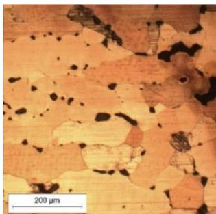
Figure 2. Microstructure of the CuSn6Pb4 reference alloy.
