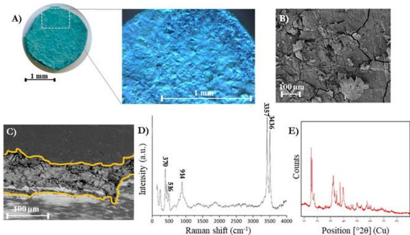
Figure 4. Obtained results on CuSn4 alloy sample brushed with NH<sub>4</sub>Cl solution 33 wt% for 1 day. In particular, A) high-quality image of the sample and superficial enlargement, B) FESEM image of the surface morphology, C) FESEM image of sample section, D) Raman spectrum and E) XRD diffractogram.
