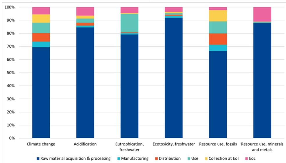
Fig. 3. LCA results for the baseline PMSM.
