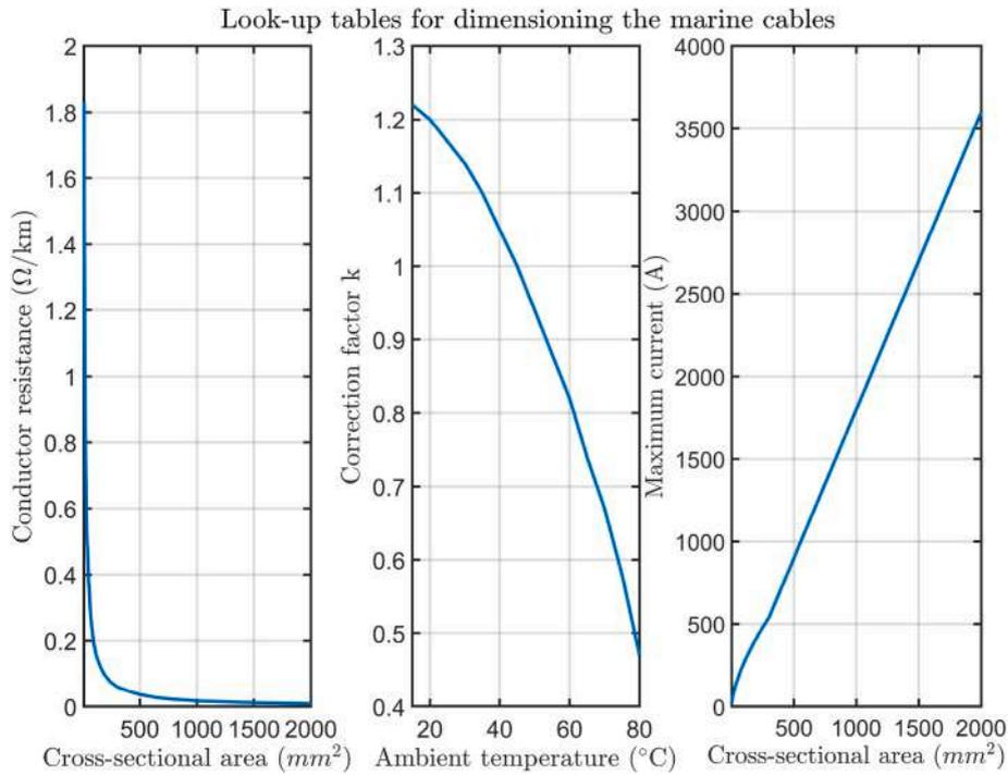
Fig. 6. Look-up tables for dimensioning the marine cables.
