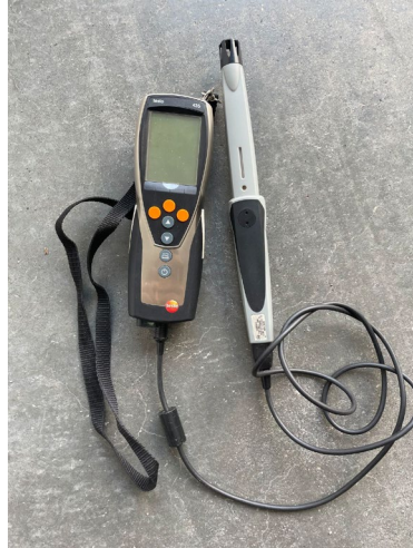
Fig. 2. The Testo 435 detector. (Source: Authors.)
