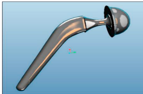
Fig. 7 Charnley prosthesis prototype
