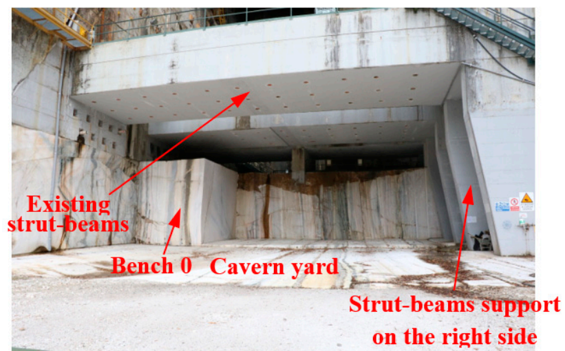
Figure 2. Detail of the first exploitation cut below the beam-struts where the marble extraction works are currently concentrated in the entrance zone of the cavern (Cava Madre of Candoglia).
