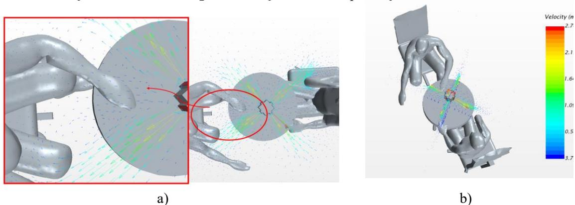
**Figure 3.** Velocity vectors a) on the horizontal plane, b) on two vertical planes intersected with Bio-stopper outlets
