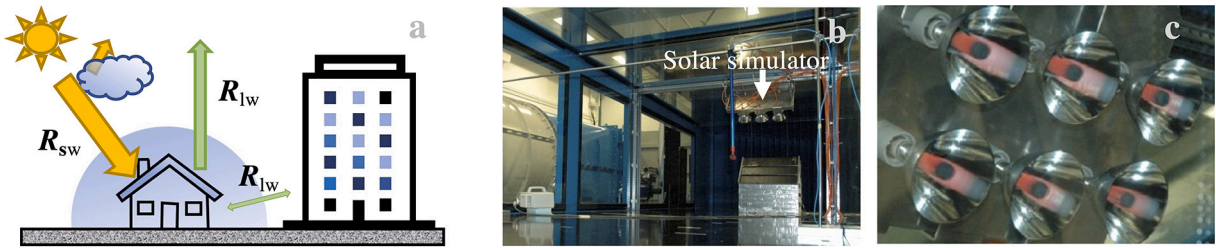
Fig. 2. (a) Schematic of short- and long-wave radiation over building surfaces, (b) wind tunnel setup for measurements, and (c) solar simulators used in a wind tunnel (Mirzaei and Carmeliet, 2015).
