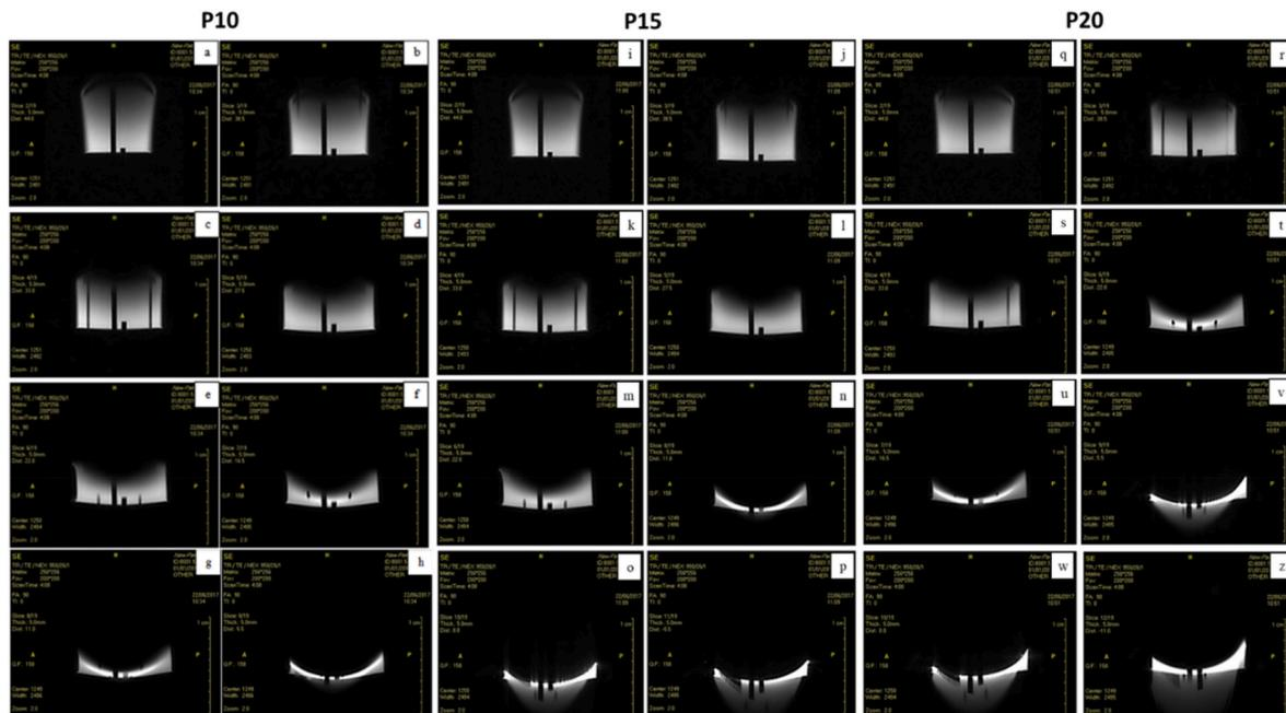
Fig. 11. Spin-echo scans of the phantom containing the contrast liquid and the composite bone cement samples weighted on  $T_1$ , in different sections, from surface to the central one (P10: a-h; P15: i-o; P20: p-z).
