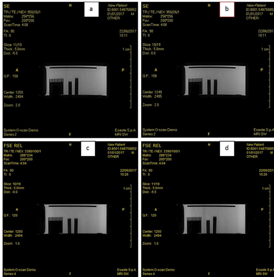
Fig. 10. Spin-echo scans of the phantom (central sections) containing the contrast liquid and the plain Palamed® samples weighted on T<sub>1</sub> (a, b) and T<sub>2</sub> (c, d).
