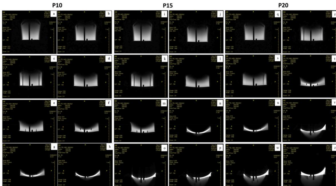
Fig. 11. Spin-echo scans of the phantom containing the contrast liquid and the composite bone cement samples weighted on T<sub>1</sub>, in different sections, from surface to the central one (P10: a-h; P15: i-l; P20: m-r, s-z).
