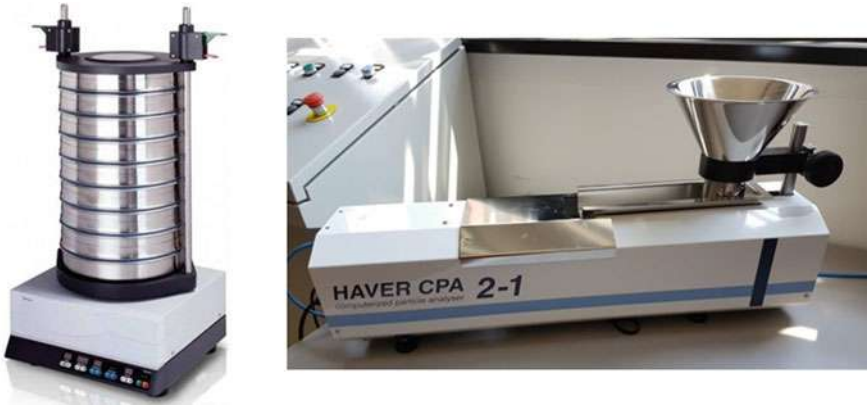
Fig. 3 Analytical vibrating sieve on the left (Retsch) and optical computerized particles analyzer on the right (CPA 2-1 of Haver & Boecker)
