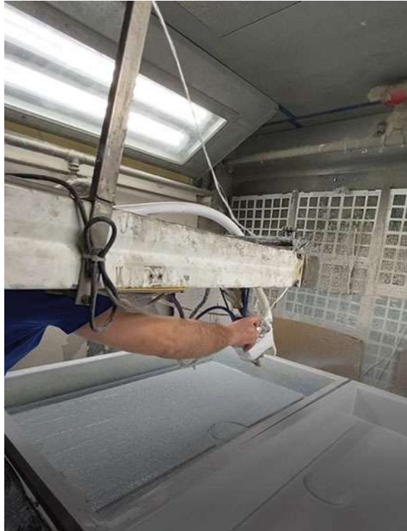
Fig. 6 Modified device for spraying granules
