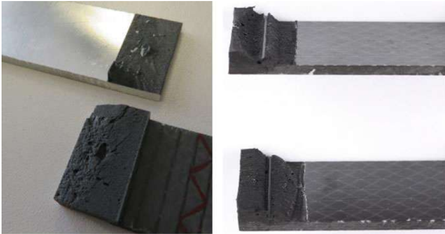
Fig. 6 Separated parts using of TEPs (left) and using electric energy (right)
