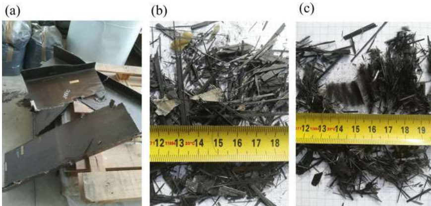
Fig. 13 a Waste Ref. F2, b Grinded waste, c Obtained short rCF
