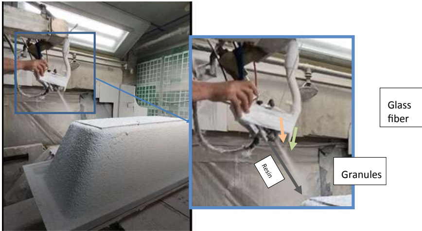
Fig. 7 Production of bath tub demonstrator
