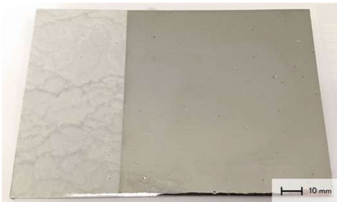
Fig. 3 UP-based sample before (on the left) and after the chrome coating using (on the right) UV-curable primer
