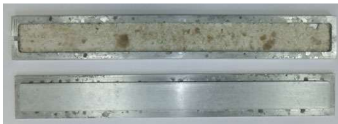
Fig. 10 Reinforcement part made of rGFRP to be used in the center area of a ski
