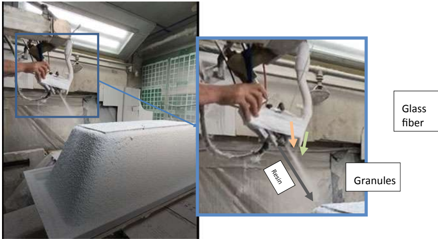
Fig. 7 Production of bath tub demonstrator
