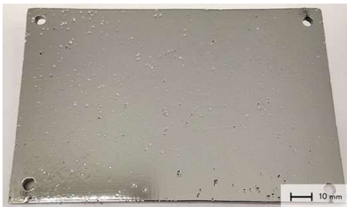
Fig. 4 UP-based sample after chrome coating using solvent-based acrylic primer
