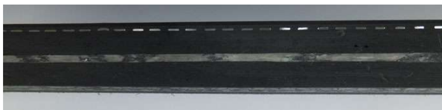
Fig. 12 Crosscut of a ski with the reinforcement in the center area made from rGFRP
