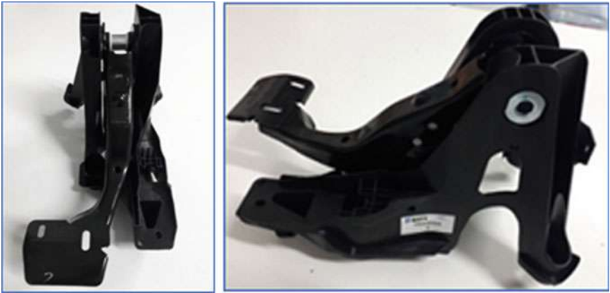
Fig. 7 Pedal bracket prototype ready for validation test
