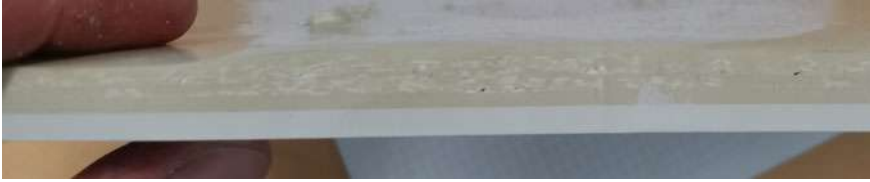
Fig. 5 Cross section of shower tray with rGFRP
