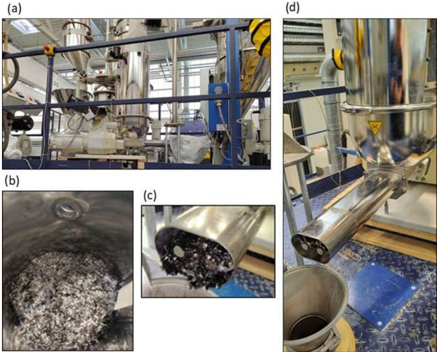
Fig. 10 a Specific dosing unit for fiber strand b rCF in the hopper c rCF being dispensed by the twin screws of the feeder d Detail of the dosing unit and the funnel of the IMC machine
