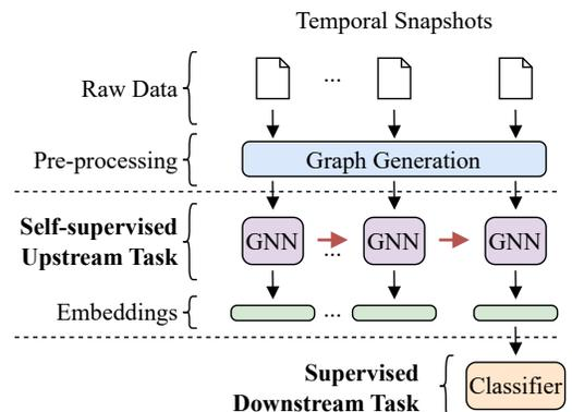
Figure 1: 2-stage DL pipeline for classification tasks.
