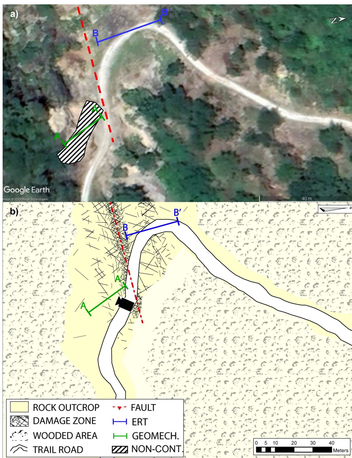
Fig. 3 a Aerial view of the Rinconada Fault (red dashed line) site. b Planimetric sketch of the Rinconada Fault site and executed surveys. The black camera represents the shooting point of the
