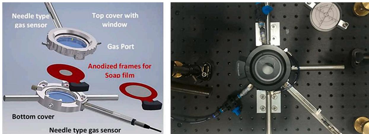
**Fig. 4.** Experimental platform for the characterization of the soap film permeability to gases: exploded rendering of the different components of the platform (left), and the set-up of the manufactured product (right). Note that, for the experimental testing, the connection between the two chambers is removed so that gas diffusion between the two compartments be only possible through the soap film (see also Fig. S10).
