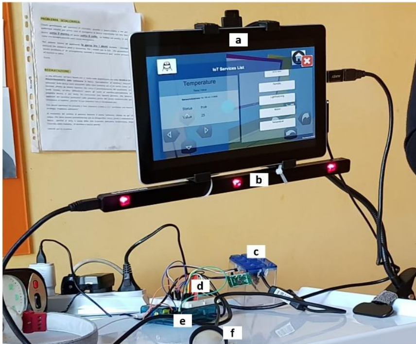
Figure 6. System Prototype composed of a main PC, (a) a Tablet PC with the Patient App, (b) Eye-Tracking device (Tobii Tracker), (c) a Relay single board, (d) a Breadboard with PIR Sensor and DHT11, (e) a Raspberry Pi 3 Model B+ and (f) a Lamp [3].
