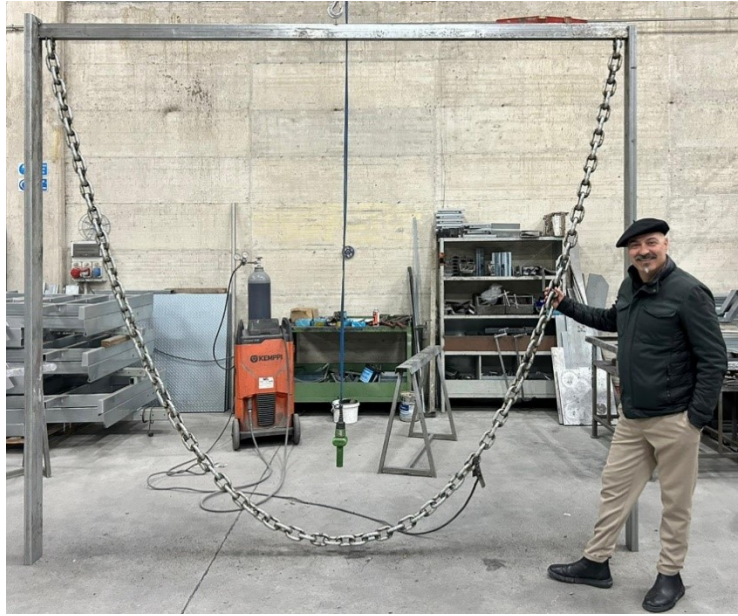
Fig. 1: The catenary arch obtained after the welding of the joints.
