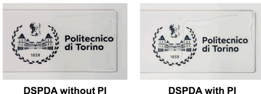
Fig. 8. Images of photocured DSPDA coatings (approximately 10 \mu m thick) on glass slides.
