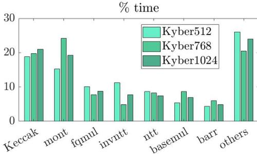
Fig. 1. CRYSTALS-Kyber profiling
