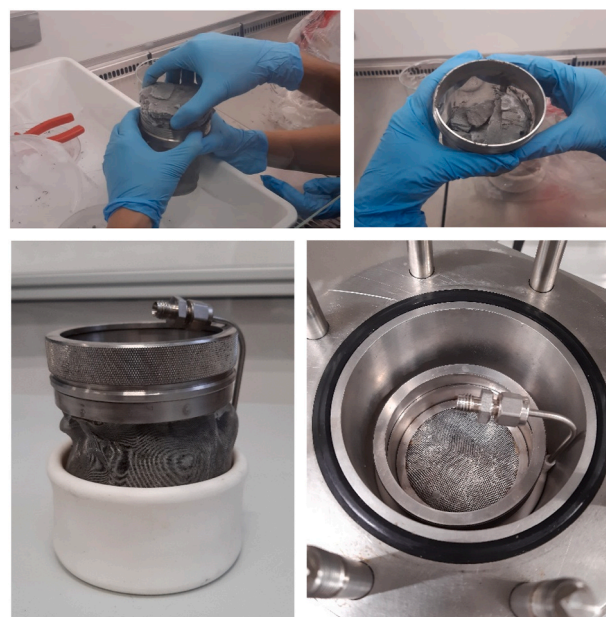
Fig. 2. Rock inoculum preparation and its positioning inside the vessel.
