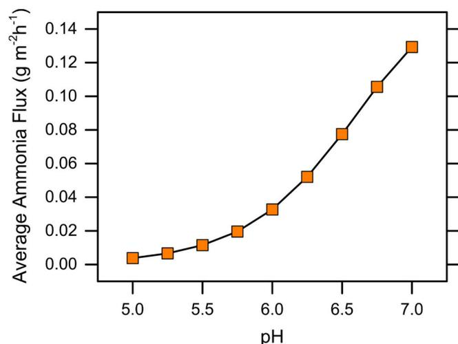
**Fig. 8.** Effect of feed pH on the average (between 0 and 90 % water recovery) ammonia flux obtained with the (orange squares) model. The same operational conditions were set in the model, i.e., the initial feed composition is reported in Table 2, the feed and distillate temperatures were set at 55 °C and 25 °C, respectively, and the cross-flow velocity was 0.068 m/s.
