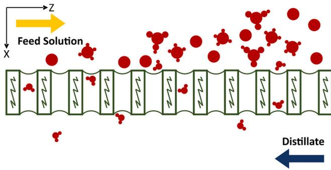
Fig. 2. Schematic diagram of direct contact membrane distillation configuration. In this work, the  $z$  axis refers to the feed and distillate cross-flow direction while the water flux occurs across the membrane in the  $x$  direction.
