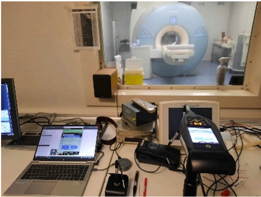
FIGURE 2 Acoustic measurements setup during calibration in the MRI control room.
