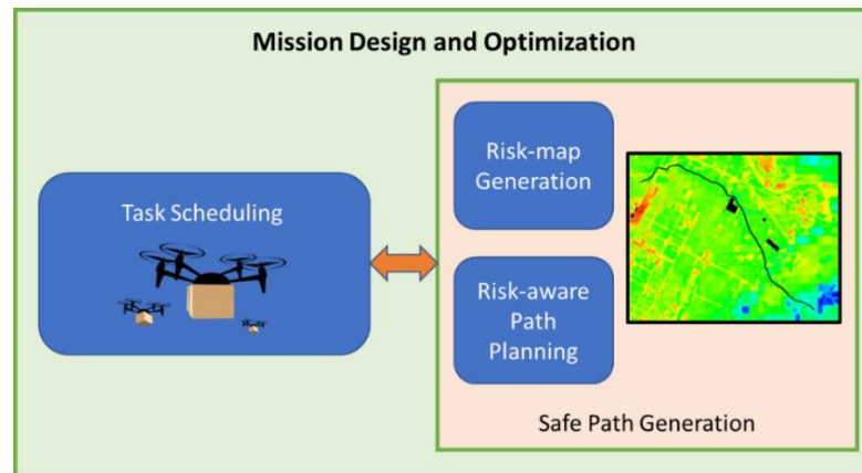
Figure 4: The main architecture of the Mission Design and Optimization tool
