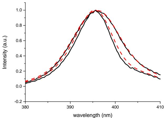
Fig. 5. In dashed red the spectra of radiation from two LEDs with the maximum at 396 nm and 397 nm. In solid black the same LED radiation measured with a reference spectrophotometer.
