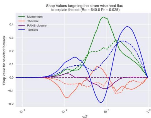
Fig 3. Shapley values obtained for DNS (solid line) and RANS (dashed line) input data.
