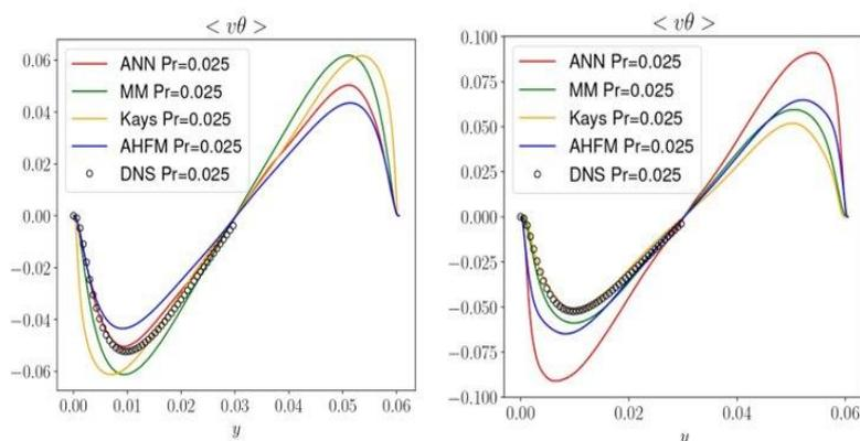
Fig.1 Comparison of heat flux predictions when the thermal models are combined with the RSM (left) and the k-epsilon model (right).
