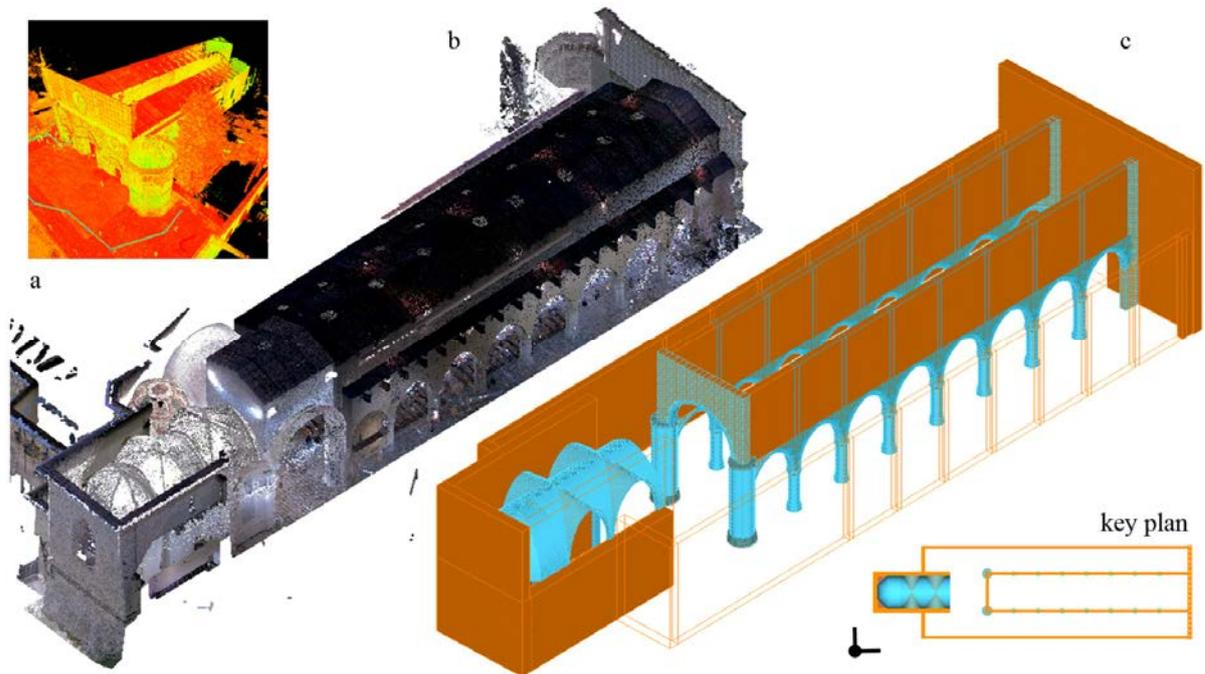
Figure 4: Laser scanner survey of the Basilica (a), processed point cloud (b), and developed numerical model (c)
