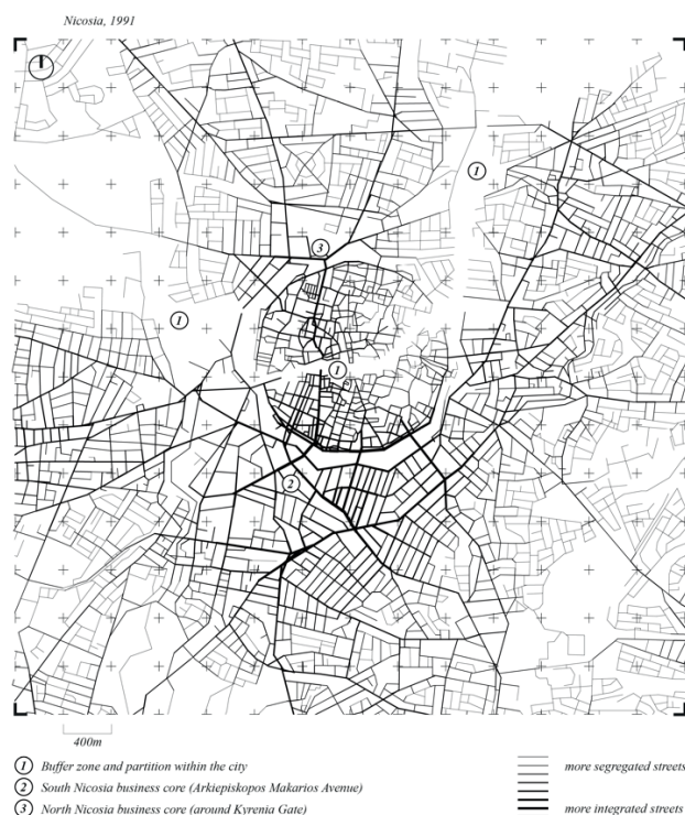
Fig. 2. Axial map of the degree of integration of each road in Space Syntax in 1991 (elaboration of the author)
