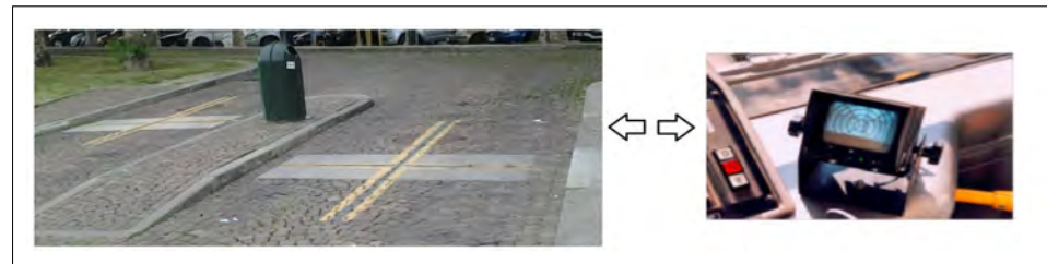
Figure 19. System used to position the bus correctly. On the left, the inductive charging station at the terminus in Corso Cairoli, Turin (IT): the black and yellow crosses are painted to correspond to the buried primary coils. On the right, the real-time video adopted by the driver to park the bus in the correct position.
