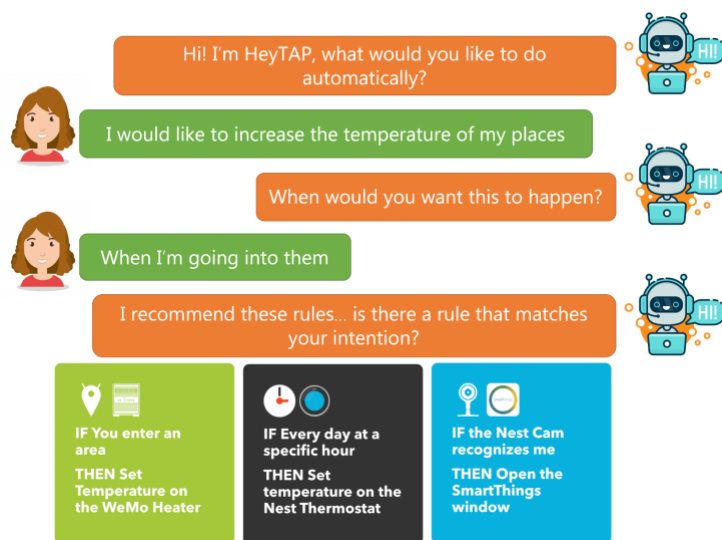
Figure 6.3.5. HeyTAP 2 is a chatbot for defining IF-THEN rules that implements a preference-based feedback approach: it iteratively collaborates with the user to get a personalization intention and refine recommendations. Image taken from the original paper.
